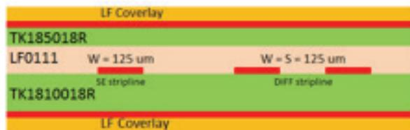
Simply replacing AP with TK in a standard flex can deliver flexibility benefits. Both stackups shown are 50 Ohms Single Ended and 100 Ohms Differential, but the TK stackup is significantly thinner and has much lower modulus than the standard flex stackup. LF bondply can be used for short lengths or longer lengths at frequencies less than 2 GHz.
