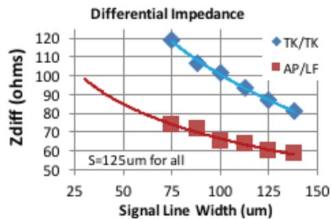
Graphs above show the impedance at different line widths for the two constructions. This shows the real advantage of lower Dk for making controlled impedance circuits. To achieve standard impedance targets at achievable line widths the AP/LF constructions would need to have a thicker dielectric between the two ground planes.
